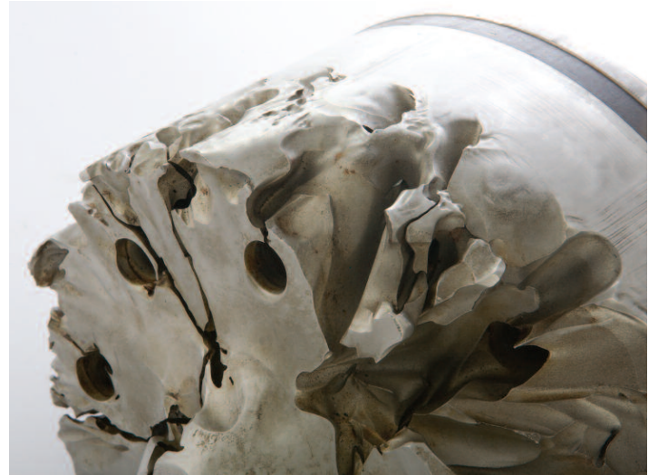
Fully stellited cage guided trim after two weeks operation
